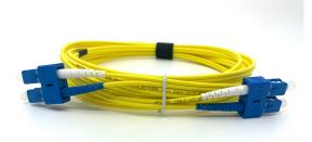
The duplex fiber patch cord is OS2 with 3 mm jacket. It is LSZH rated and its terminated with SC fiber optic connector on both ends.
